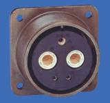
Insert pattern 28-5 with (2) size 4 RADSOK sockets and standard contacts: (1) size 12 and (2) size 16
