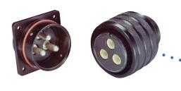
The Amphe-Power Series consists of three of the time-tested and reliable families of Amphenol Industrial Connectors, all of which are MIL-C-5015 styles, medium to heavy duty cylindricals. These series, enhanced with RADSOK sockets, can now handle up to 150% higher amperages. Current Amphe-Power product line supports from 50A to 1000A continuous duty.
