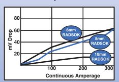
The RADSOK design provides lower millivolt drop at an increased current load. This allows users to increase the current load per circuit while reducing the total number of circuits in the application, resulting in lower overall costs.
