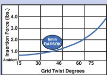
RADSOK contacts can be tailor designed to meet the customer's requirements. By varying the degree of twist, the insertion/extraction force can be customized.
