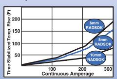
Although actual data may vary with the style of connector, typical thermal rise data after 500 cycles of durability is:
